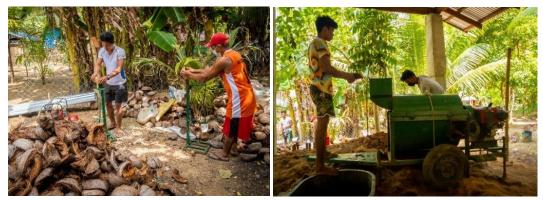
Figure 16. Male BFA members dehusking the coconuts (left) and feeding the husks soaked overnight into the decorticating machine.
