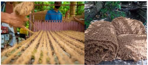
Figure 18. BFA members operating the weaving machine (left) to produce geonets (right) from twined coco coir.
