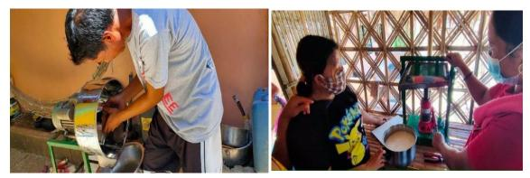
Figure 22. BFA members extracting coconut meat using the electric grater (left) and coconut milk using mechanical presser (right).
