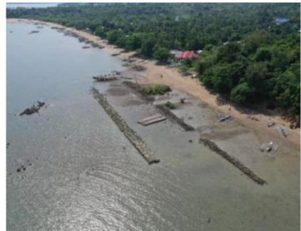
Figure 4. Drone shot of the semi-permeable living breakwater in Purok Malipayon in Loong (Site 1).
