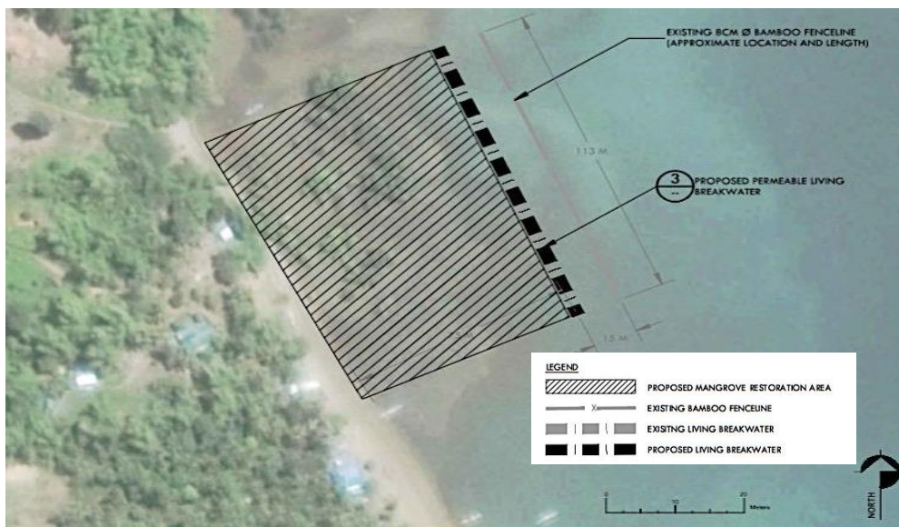
Figure 2. Green-grey infrastructure design for Bacjawan Norte.
